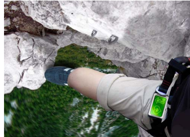
Figure 2: The smart harness - the harness provides information on the climbing partner
