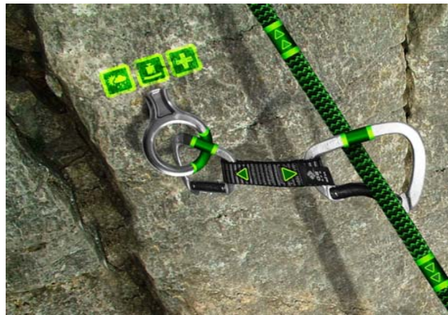
Figure 3: The smart hooks built up a geosensor network to collect and dispread information.
