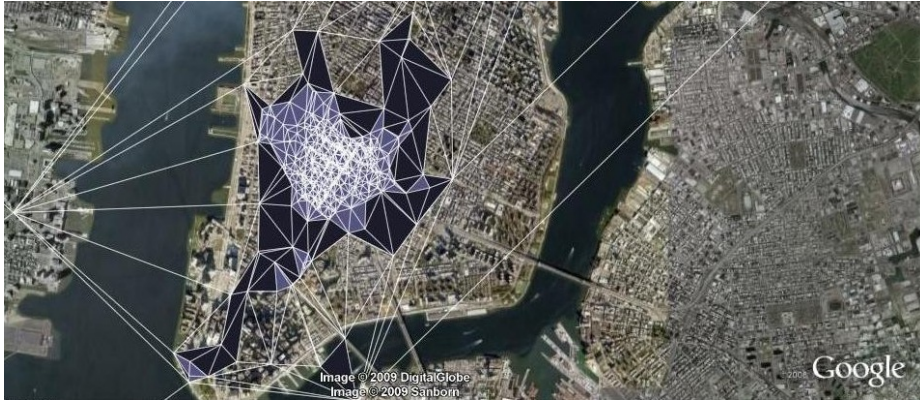
Fig. 2. Cluster graph after the Delaunay triangulation for the place name Soho . The screen shot shows the clustering result depending on the edge length threshold: A small value results in several small clusters shown in blue. When the threshold increases, the fragments starts to join to the large black cluster.
